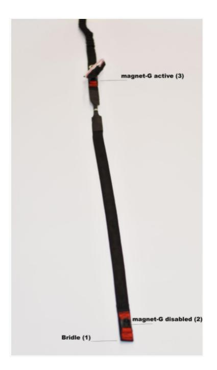
Attach the main bridle (1) to either the left or right main hang point karabiner. The bridle should be attached to the other side which you are going to do spiral: for example, If you wish to spiral to the right, the bridle should be connected to the left side in your harness.
