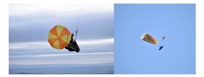
G-Killer is a small parachute that significantly reduces G-forces during descent in a deep spiral. Its use helps to achieve a higher sink rate with fewer turns.
